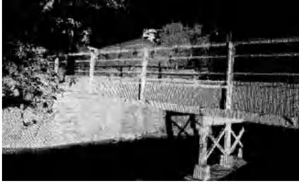
Fig. 7. Terrestrial laserscan of a bridge gives 3D information
